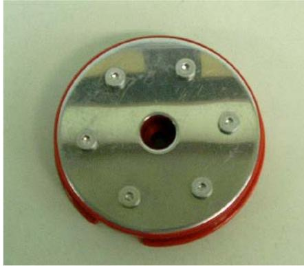
5. Pad holder fixed plate. Wipe it with a soft cloth that's been wet with water or window cleaner.
