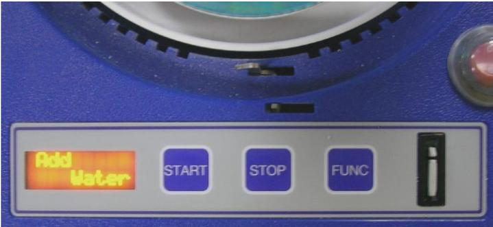
**Add water to the Water Bottle, and then press any button on the Operation Panel to clear the alert indication.**
