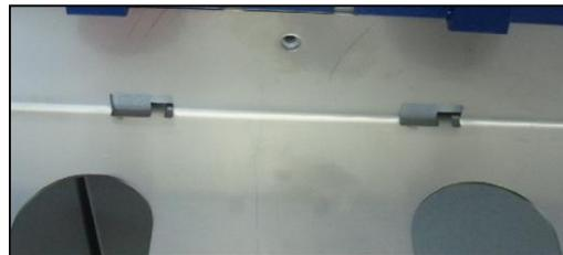
3. Secure the Bottle Holder by re-installing and tightening the Bottle Holder Thumb Screw.
