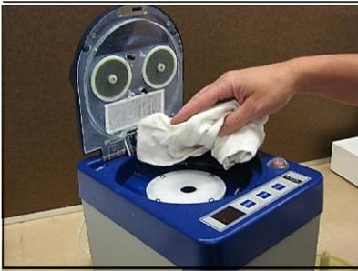
5. Spray the platen table assembly with glass cleaner and scrub with a toothbrush to clean it.
