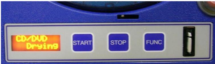
6. After finishing the disc drying process, the Lid opens automatically, and then the Platen Table stops.
