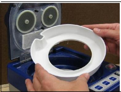
7. When you put the platen table assembly back into the machine, align the groove in the base with the pin on the motor spindle.
