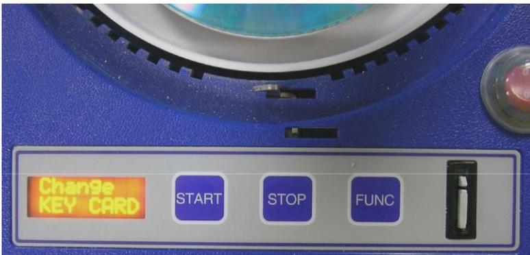
Turn OFF the Main Power Switch, exchange the KEY CARD (see page 9 for removal tips)
