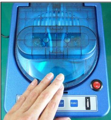
**Caution! Closing the Lid without a disc on the Platen Table may cause pad damage.**
