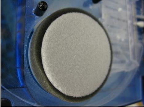
✓ Pad installed **CORRECTLY**
