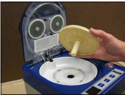
2. Take the polish tray out of the machine and wipe it with a damp cloth. You may also wash it in the sink, if needed.
