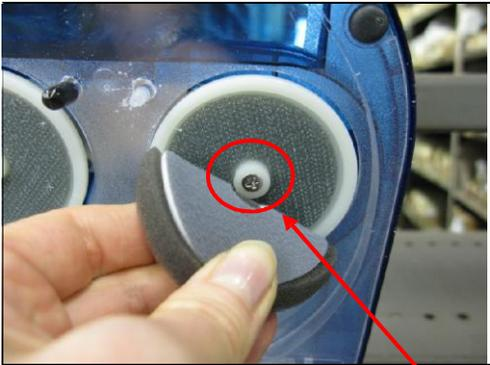
Bend the Pads lightly with fingertips, and fit the hole in the middle of the pad over the center pin of the Pad Holder
