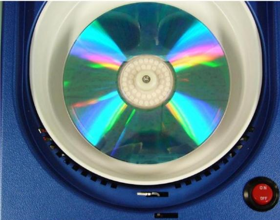
★ **IMPORTANT: Place the disc so that the side to be repaired faces upwards.**
