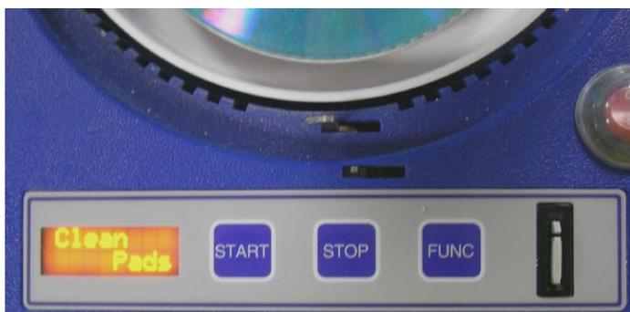
Exchange the pads for a clean dry pair and **press any button on the Operation Panel to clear the message.**
