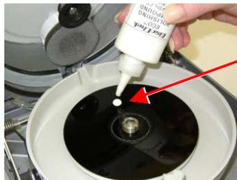
Place a small dab of compound at the 12 O’clock position for the second part of stage 1.
